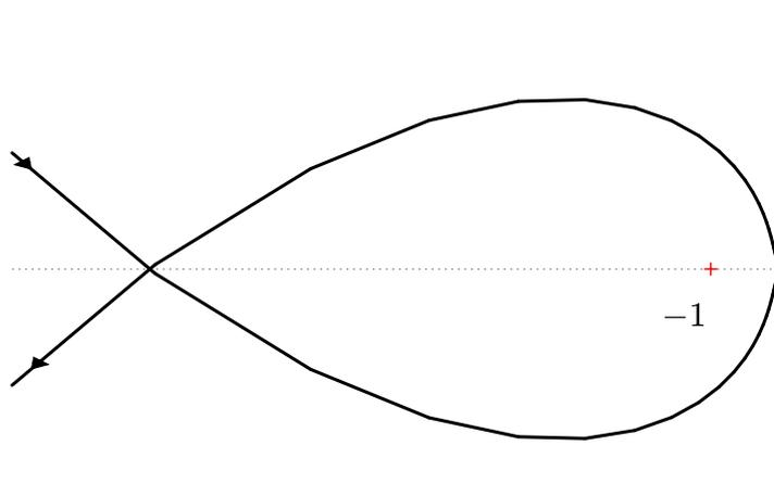
It ends at origin with arriving angle  $-180^\circ$ . One **possible** Nyquist plot (generated using  $G(s) = \frac{1}{s(s-1)} 100 \frac{\frac{s}{10} + 1}{\frac{s}{100} + 1}$ ) is shown above.
